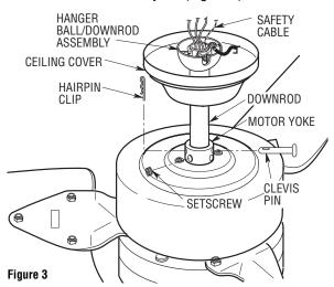
6. Align the clevis pin holes in the downrod with the holes in the motor yoke. Install the clevis pin and secure with the hairpin clip (Figure 3). The clevis pin must go through the holes in the motor yoke It is critical that the clevis pin in the motor yoke is properly installed and the setscrews securely tightened. Failure to verify that the pin and setscrews are properly installed could result in the fan falling.
